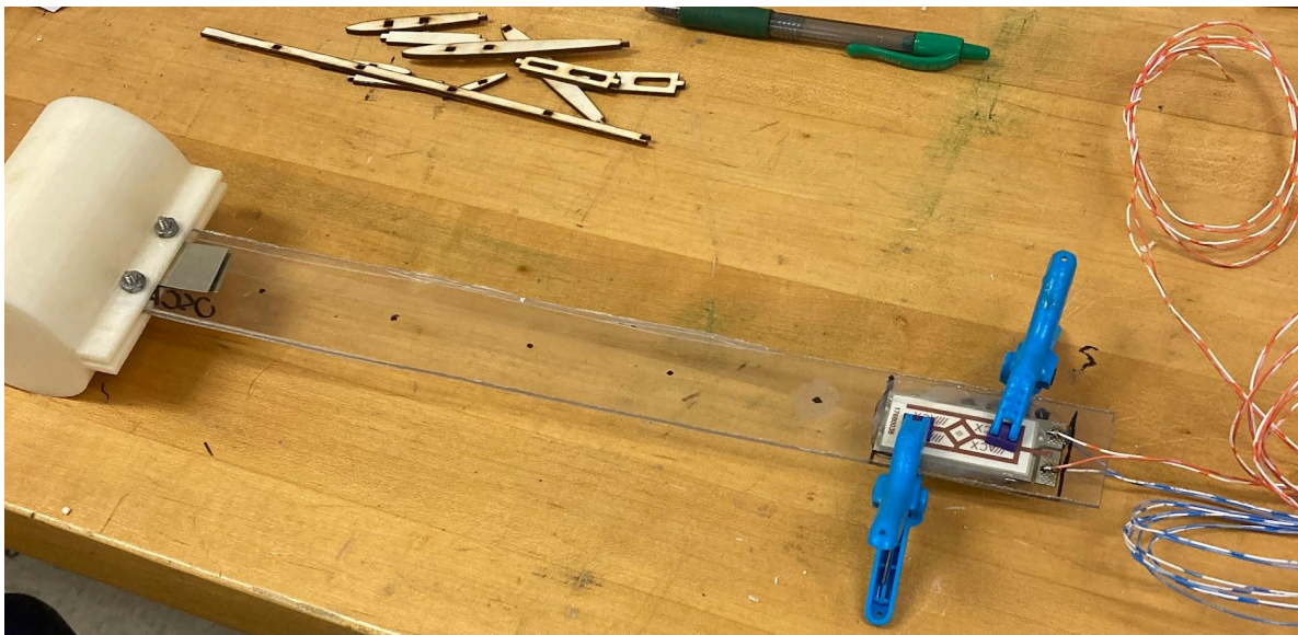
Figure 10: Piezo strips attached to Beam
